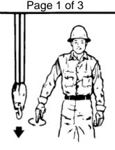
LOWER. With arm extended downward, forefinger pointing down, move hand in small horizontal circle.
