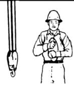
TRAVEL (Both Tracks). Use both fists in front of body, making a circular motion about each other, indicating direction of travel, forward or backward.
