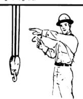
MOVE SLOWLY. Use one hand to give any motion signal and place other hand motionless in front of hand giving the motion signal. (Hoist slowly shown as example.)
