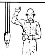
TRAVEL. (One Track) Lock the track on side indicated by raised fist. Travel opposite track in direction indicated by circular motion of other fist, rotated vertically in front of body. (For land cranes only.)
